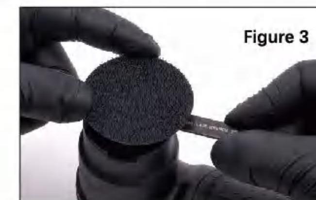
Insert wrench into flat square shaft, and then rotate polishing pad. This way you can easily install all the polishing heads.
